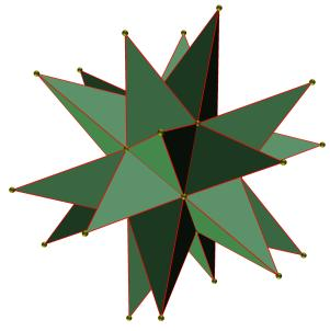
The construction is logical and easy to implement using Asymptote. First define the twelve points of the icosahedron, then use these points to define the twenty faces and, finally, create a function that will erect a pyramid on (i.e., stellate) each of these faces. Asymptote itself takes care of the projections and shading.
